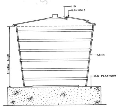
Figure 2— Typical view of open top tank
